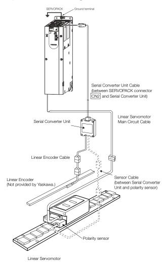
\* You can connect directly to an absolute linear encoder.
