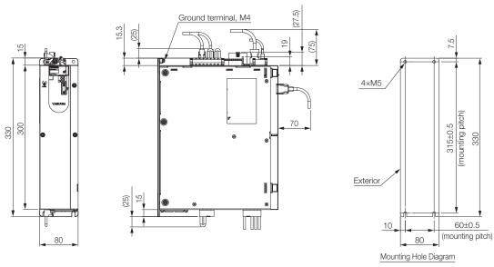
Approx. mass: SGD7S-1R9D, -3R5D, or -5R4D: 3.4 kg SGD7S-8R4D or -120D: 3.7 kg Unit: mm
